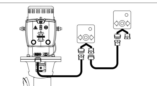
If it is found during test running that the thrust direction does not correspond with the direction switch on the control panel then the blue (no. 1) and the white (no. 4) wires on the relay must be interchanged.
